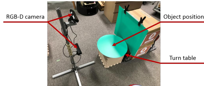
Fig. 2. Overview of proposed autonomous annotation system for YOLO.
