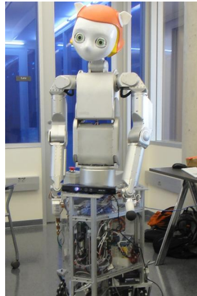
(d) Dreamer is a compliant humanoid robot used in Sentis's laboratory.
