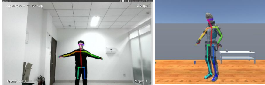
Fig. 5. CMU OpenPose skeleton detector
