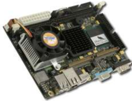
Fig 4.7 Embedded card JReX used for robot controller
