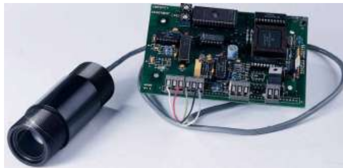
Fig.7.2 IR Sensor model OS65 used for body temperature measurement
