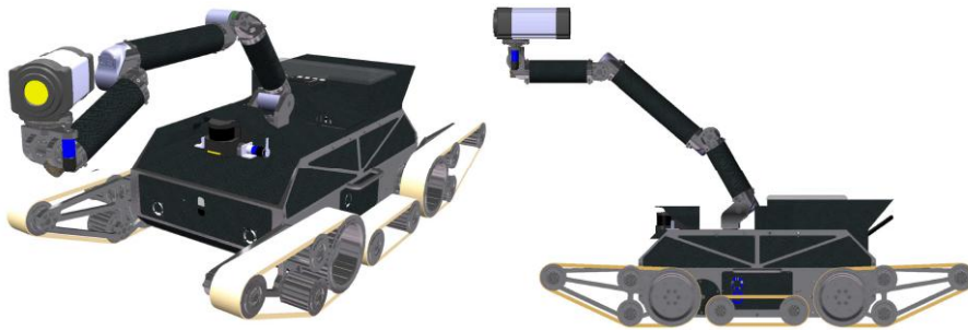
Fig. 12. Rescue-Robot Construction in CATIA
