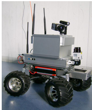
Fig. 1. Current robotic vehicle "Monstertruck".
