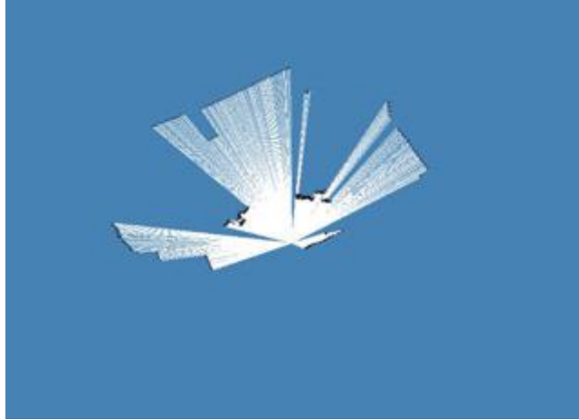
Fig. 3 Example of a map obtained by the laser sensor.
