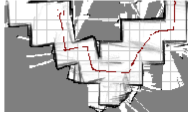
(b) Map generated from data of a rigidly coupled LRF.
