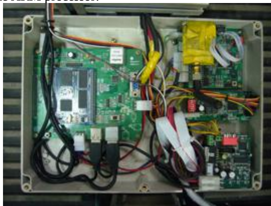
Fig. 5 The control box on the old robot
