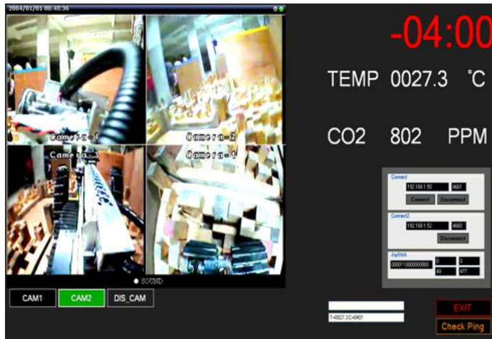
Figure 3: Operator console of iRAP_PRO illustrated the real time quad videos and information of the robot's sensors.
