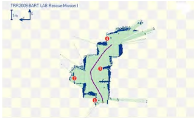
Fig. 6. Closer-Look of the Generated Map, and the Robot's Path Generated by the "Layer-Sweeping Search" Navigation Algorithm
