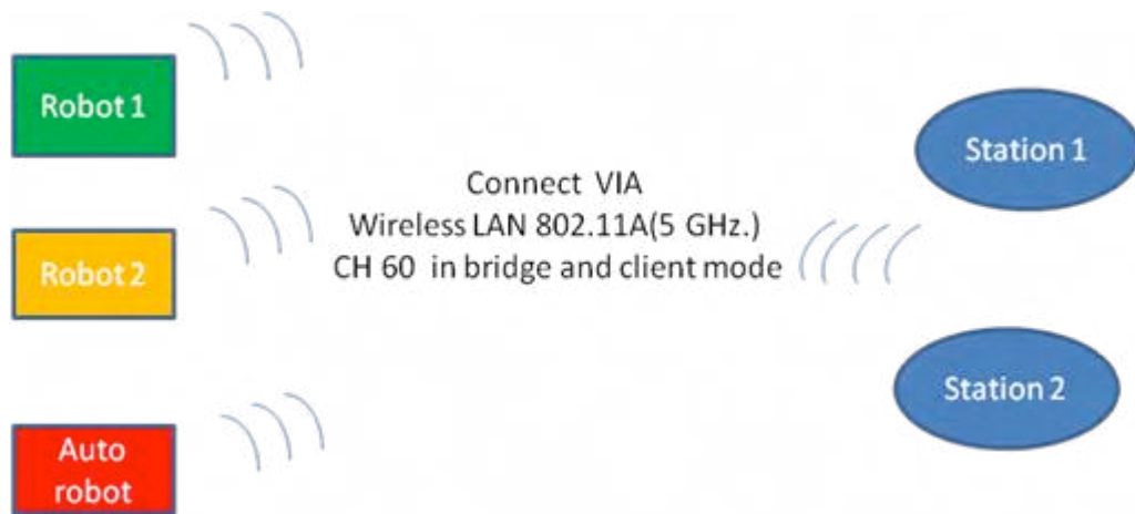
Fig. 3. BART LAB Rescue’s communication system.
