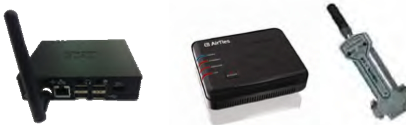
Fig. 13. FitPC2, access point and the bluetooth adapter used for communication.
