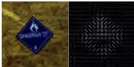
Fig. 3. Original Image (left) and histogram of oriented gradients (right).
