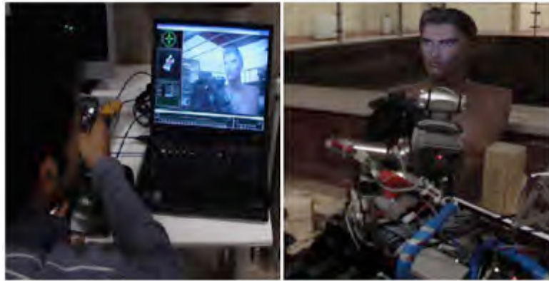
Fig. 11. Control Pack and Operator that's running the Robot and a sample of GUI
