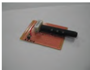
Fig. 6. RKRS custom CO 2 sensor with Heimann gas detection element.
