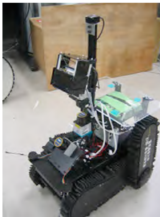
Fig. 5 HIEI(2-flipper at its rear and full autonomous robot)
