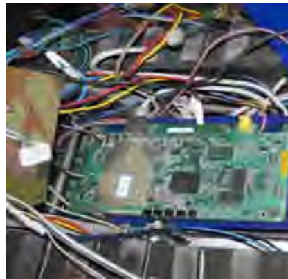
Fig. 3. Dlink Access Point Board
