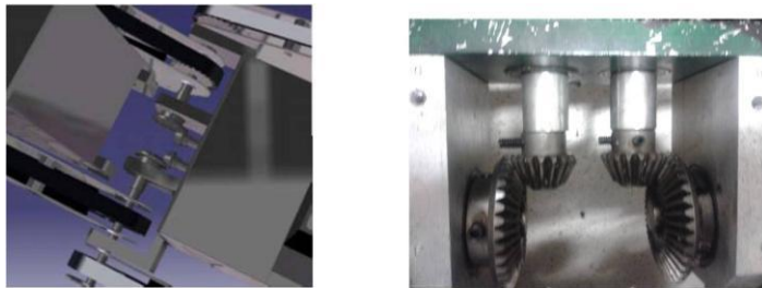
Fig. 26 Second stage of reduction with bevel gears.
