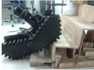
Fig. 27 Final transmission system with the two stages.
