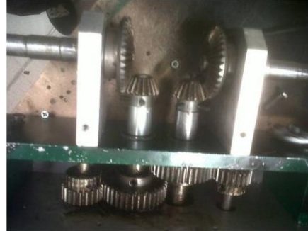
Fig. 27 Final transmission system with the two stages.
