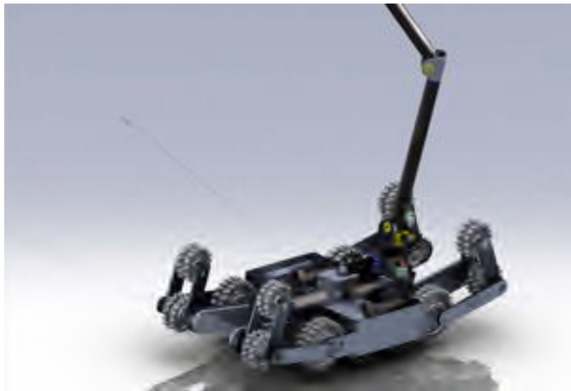
Fig. 8 QUAD-ARM robot with MANIPULATOR
