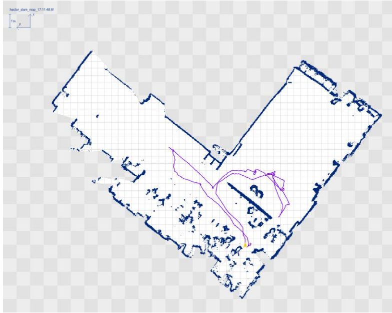
Fig. 3. Map generated by Hector SLAM using the RAPOSA-NG robot on the 8th floor of North Tower building (Instituto Superior Técnico).
