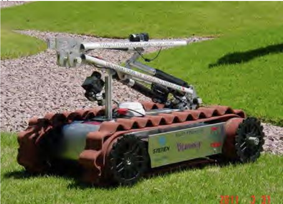
Fig. 4 Tracked wheel rescue robot IXNAMIKI ÖME: (a) design and (b) prototype.
