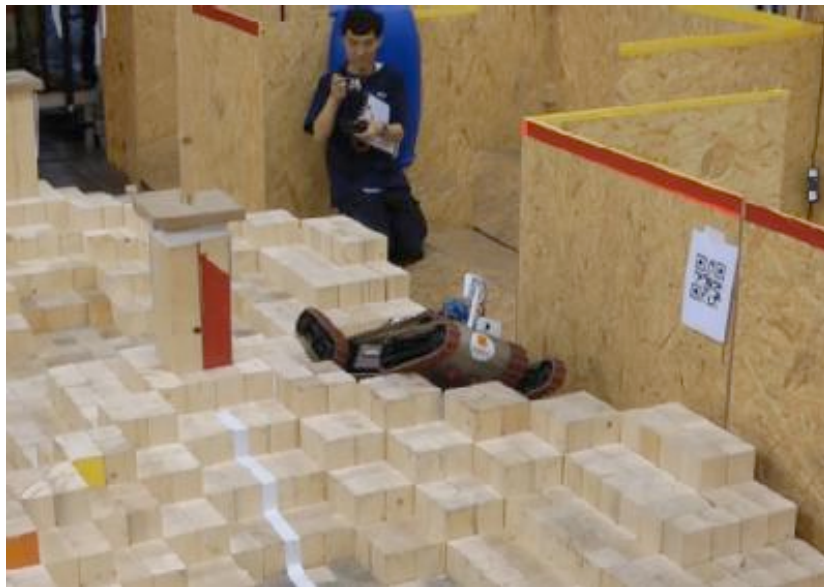
Fig. 4. WMR robot overcoming red zone step fields in the 2012 German Open Mobility Challenge.
