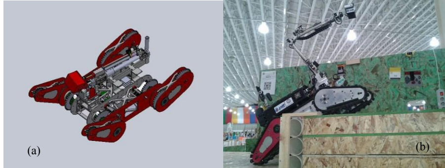
Fig. 3. (a) CAD of TeleOp V platform (b) TeleOp V in step field
