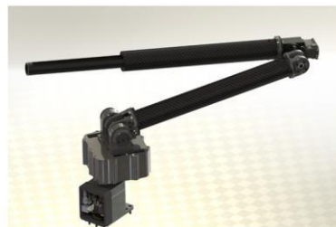
Fig. 9. New design of the 6 DOFs serial manipulator
