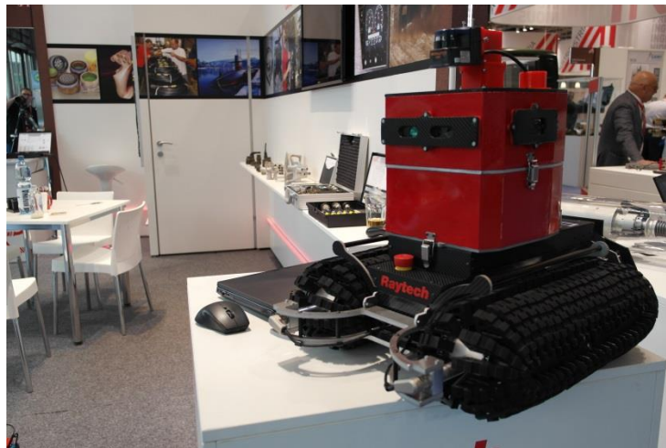
Figure 8: Red Scorpion with an Omni View Sensor System
