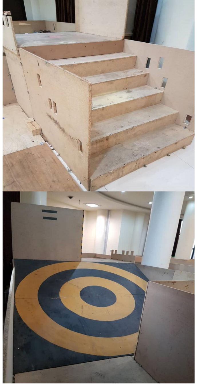
Fig. 24. Stairs and inclined planes are provided in the test arena inside the laboratory.
