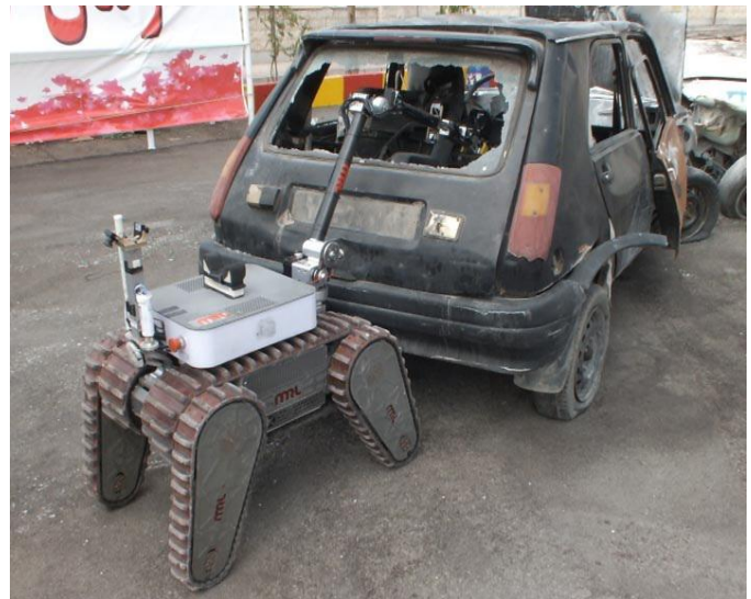
Fig. 14. Karo is inspecting insdie a car using the 6-DOF manipulator.
