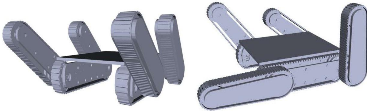
Fig. 6. 3D models of the drive part of the MARS Rescue Robot.
