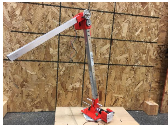
Jointed arm with rotation capabilities.
