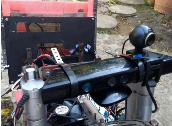
Fig. 5. Kinect sensor. (3D Map)
