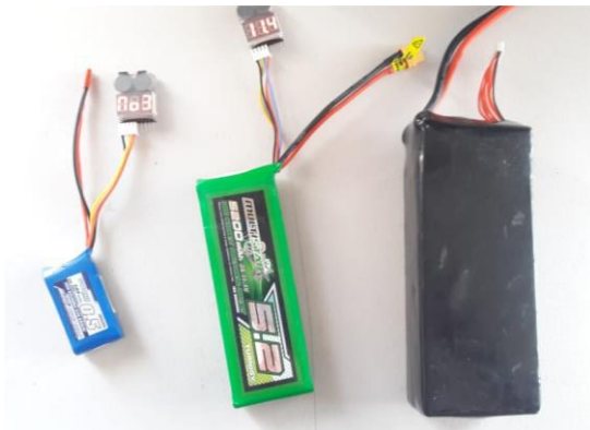
Fig.6 LiPo's used in the project.
