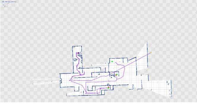
Fig. 7. The automatic map generated by iRAP ROBOT in the final round of the world RoboCup 2017 competition.
