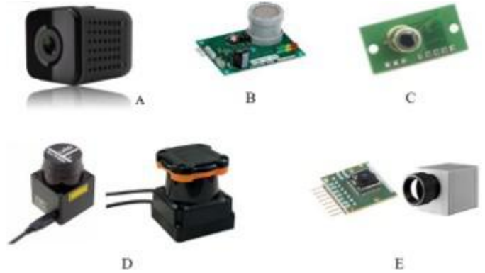
Fig. 8. Electrical components of our Robots: (A) Cameras (B) Carbon dioxide sensor (C) Heat sensor (D) Sensor Range Finder (E) Thermal sensor
