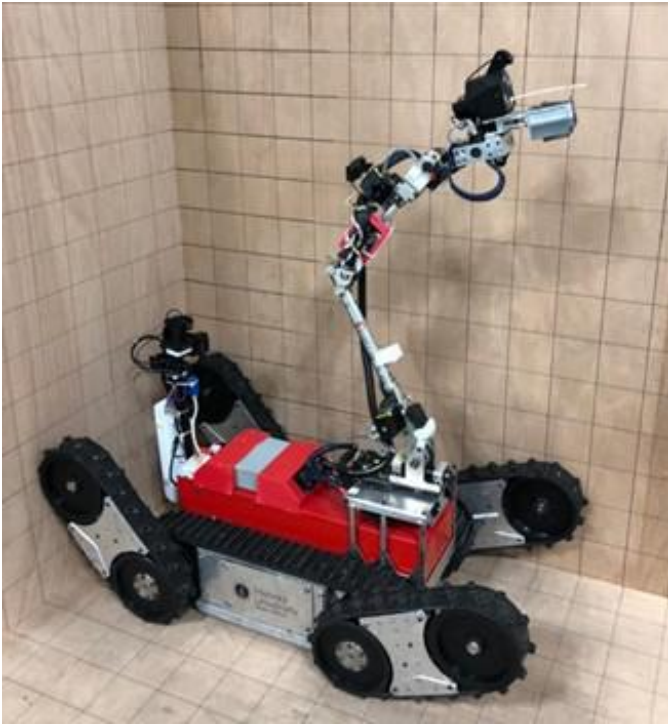
Fig. 2. TeleOp VI the previous iteration of the autonomous robot of BART LAB Rescue Robotics team
