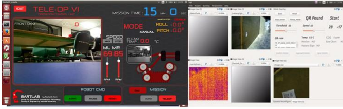
Fig. 12. Image shows the framework of (A) GUI of the tele-operative (B) GUI of the autonomous function
