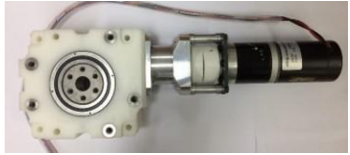
Fig. 7. New Motor-gearbox combination made by BARTLAB
