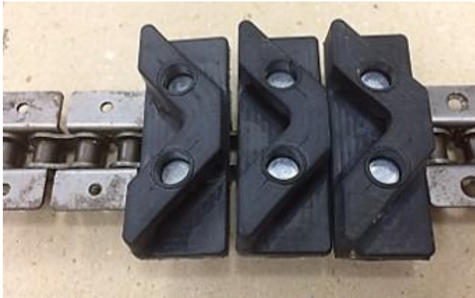
Fig. 5. Chain-rubber-equipped propulsion system the rubber teeth are designed to reduce the noise, damp impact and make a great surface contact on variety of grounds
