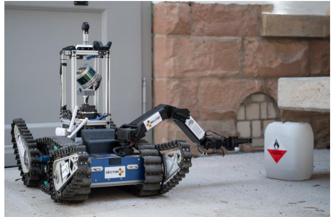
Fig. 1: Asterix rescue robot performing a visual inspection task.
