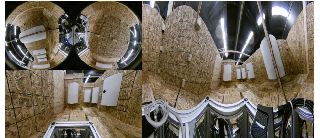
Fig. 4: Two fish-eye images are streamed from the omnidirectional camera (top-left), which are converted to perspective (bottom-left) and Mercator projection (right).
