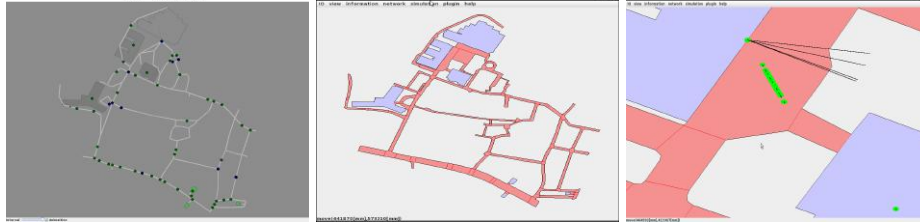
Fig. 3. Evacuation behavior simulation at disasters. [left] A snapshot of original RCRS. [middle] A new GIS viewer that deal roads with area property. [right] A snapshot of simulations that agents out of an exit of building cut across the area in front of the building.
