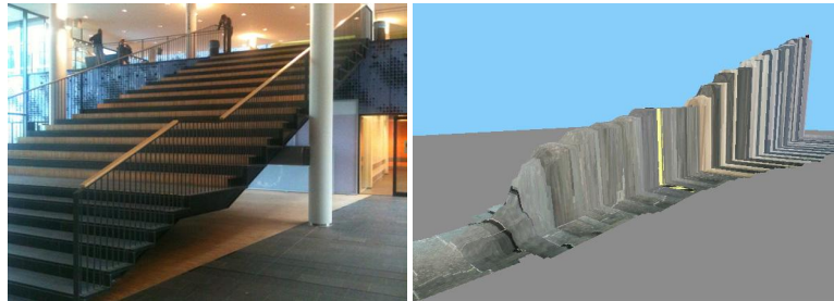
Fig. 10: Photo and map of a large stair at our university which is traversed by the AR.Drone. The depth of each step is 30cm and the height of each step is 18cm. The total height of the stair is 480cm.
