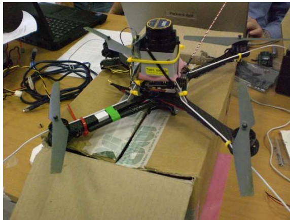
Fig. 3. Our AscTec UAV with the Hokuyo LRS installed on its top.
