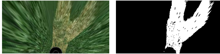
(a) Bird-eye view image from the maze. (b) Free space detected by Gaussian Mixture Model classifier.
