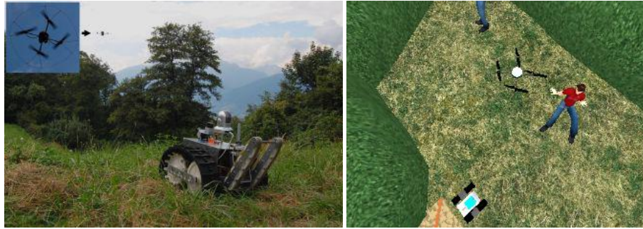
Fig. 1. Left: A Jacobs land robot cooperating with an arial robot at the European Land Robotics Trials (ELROB) 2007 in Monte Ceneri, Switzerland. In this technology evaluation event, the aerial robot has to search for hazard areas like fire in a forest, which the land robot then has to reach. Right: A simulated RugBot and AirRobot in USARSim. Much like in the real scenario, the aerial robot will allow a much broader overview of the incident area.
