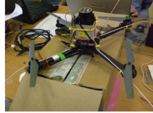
(b) AscTec UAV with the Hokuyo LRS installed on its top.
