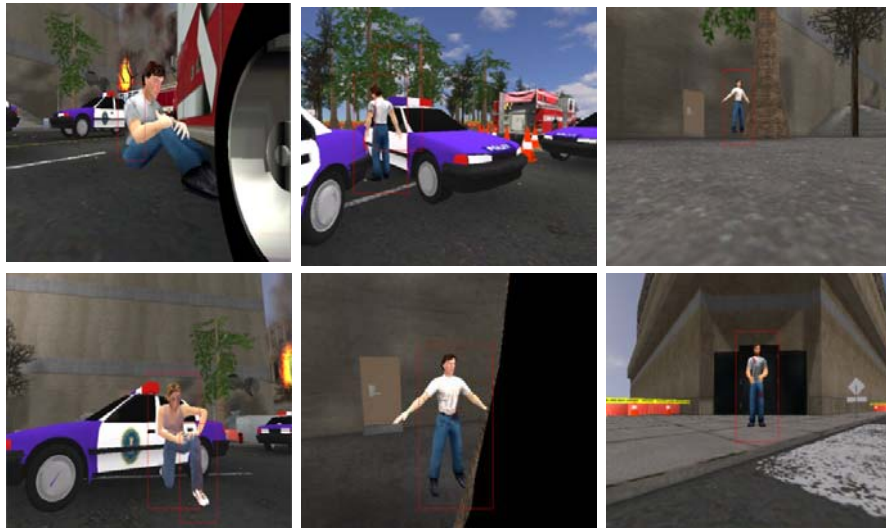
Fig. 6. Some examples of automated body detection using a HOG algorithm
