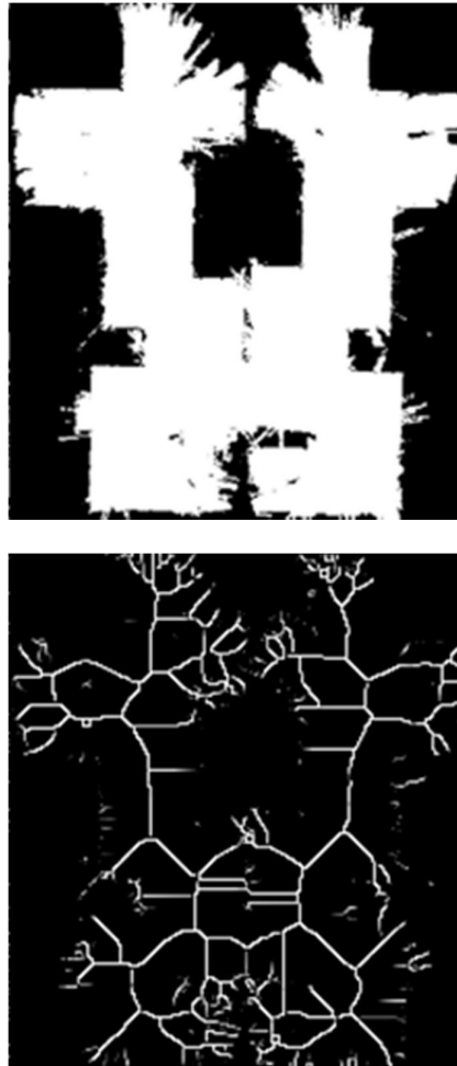
Fig. 2. Output of thinning algorithm for planning (map is related to yellow Real Rescue arena of RoboCup IranOpen)
