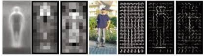
Fig. 2. HOG output for human detection [11]
