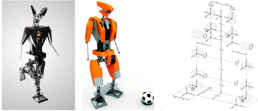
Fig. 1. Adult-size humanoid robot TULip: photo, CAD drawing and kinematic configuration in the lower body.
