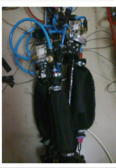
Fig 4: Pneumatic Muscles in Action in the leg area.
