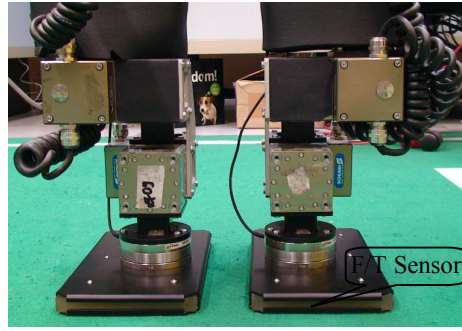
Fig. 5. Force/Torque sensors in the ankles. motion.
