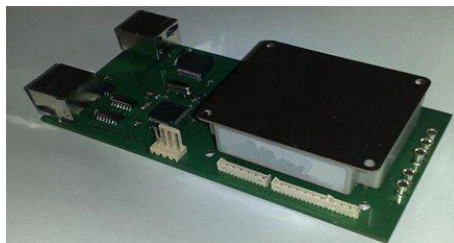
Fig. 4. ARCHIE: Brushless Motor Driver
