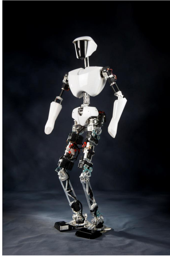
Fig. 1. CHARLI-2 (Cognitive Humanoid Autonomous Robot with Learning Intelligence)
