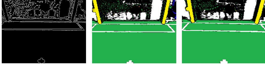
Fig. 6. Canny Edge Detector and Line Detector
