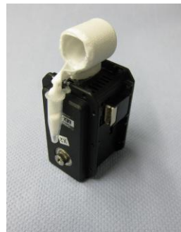
Fig. 2. Servo including wetted fleece for cooling
