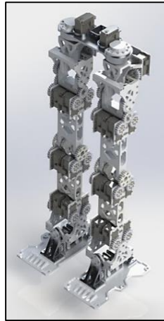
Fig 2. Artin's lower limb of next generation of IRC team robot mechanical structure (Artin).
