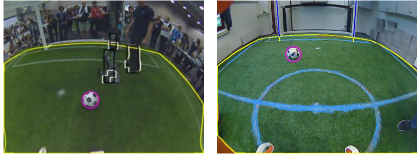
Fig. 4. Left: Visualisation of our obstacle detection. Right: A captured image with detected ball (pink circle), field lines (light blue), field boundary (yellow lines), and goal post (dark blue lines).
